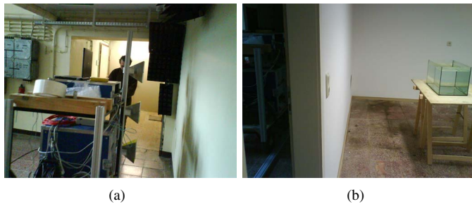
Fig. 2. The through-wall measurement scenario: (a) Radar system; (b) An aquarium filled with water.
